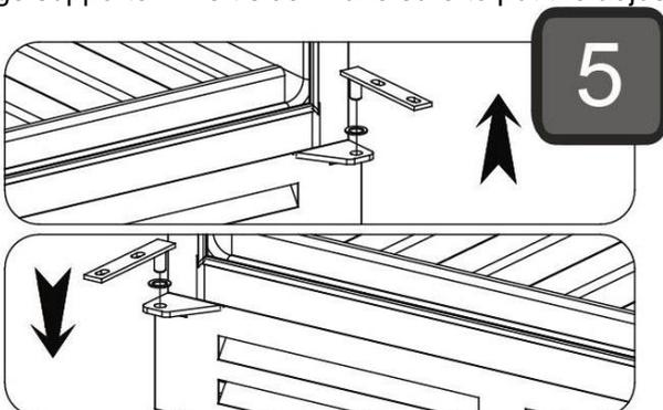
6. Locate the glass door to the designated position making sure that the door shaft enters the door hole at the left upper corner of the glass door. Install the two screws that are used to connect the left lower hinge with the glass door and tighten them before the door is leveled. Then remove the handle from the left side and install it on the right side of the door.
