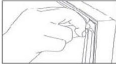
**CAUTION:** Do not over-tighten the screws as this may cause damage to the handle or to the stainless-steel door. Carefully press the door gasket into its original position.
