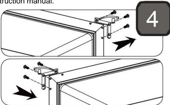
5. Remove the lower hinge supporter with the adjusting washer from right side. Install the lower hinge supporter in left side. Make sure to put the adjusting washers at the designated position.
